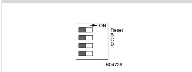
The reset switch is set to 'ON' for approx. ½ s, causing the station to load the user data from the EPROM and to start operation under defined starting conditions.
