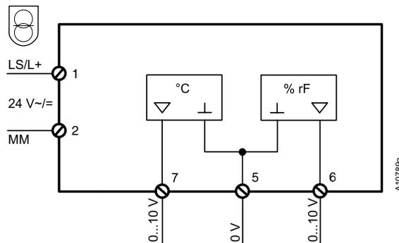
The power supply (pins 1 and 2) and the analogue outputs (pins 5 and 7) are electrically isolated from each other.
